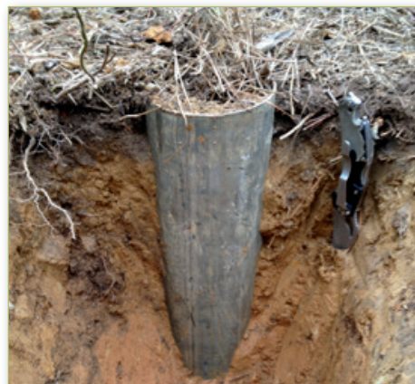
Figure 8.1. Right: Root-severing core installed at the Virginia Tier III site. Left: Root-severing core being excavated. Photos by Brett Heim.
