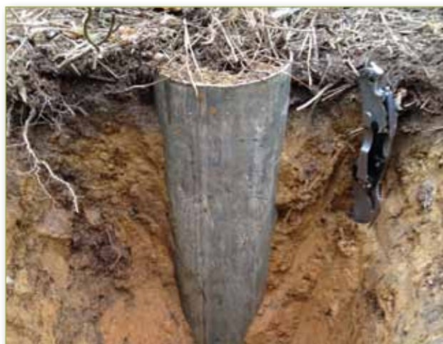
Figure 4.1. This picture shows a root exclusion core being excavated after a 90-day installation so that roots can be collected for analysis. Photo by Brett Heim.
