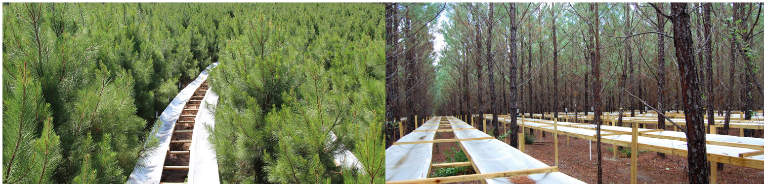
Throughfall exclusion structures at the PINEMAP “throughfall exclusion x fertilization” sites (left: McCurtain County, OK; right: Taylor County, FL).
