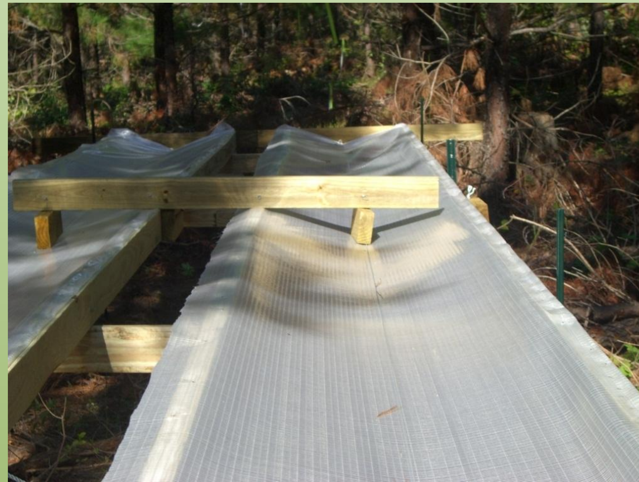
Figure 1. Throughfall exclusion in Pinus taeda plantation
