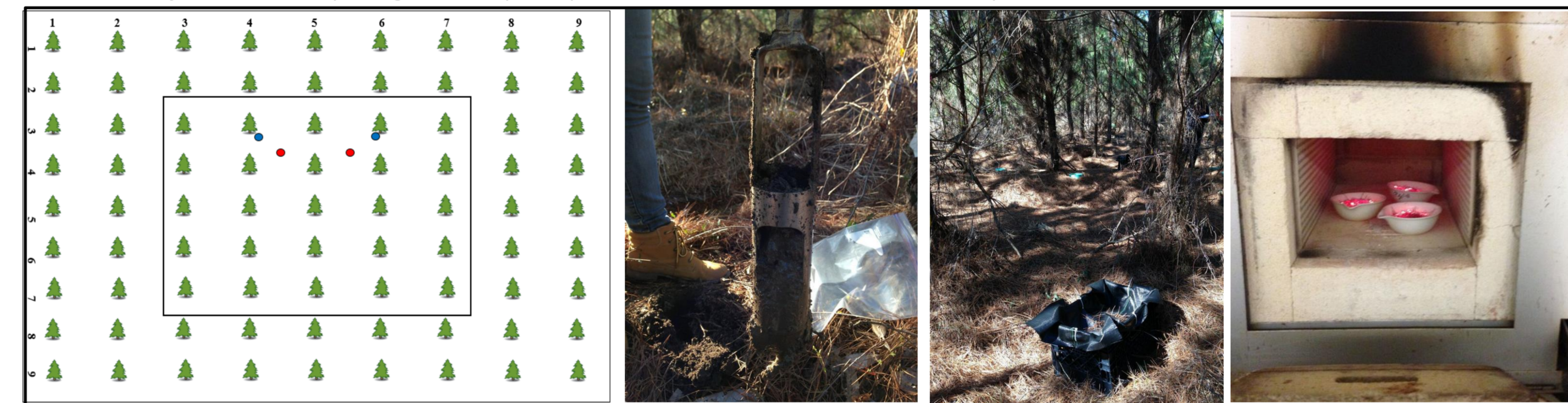
Figure 3. Locations of soil C sampling; auger used for sampling, litter fall collector in plot; analysis of the ash content in a muffle to evaluate the amount of mineral soil present in the samples, after being sieved.
