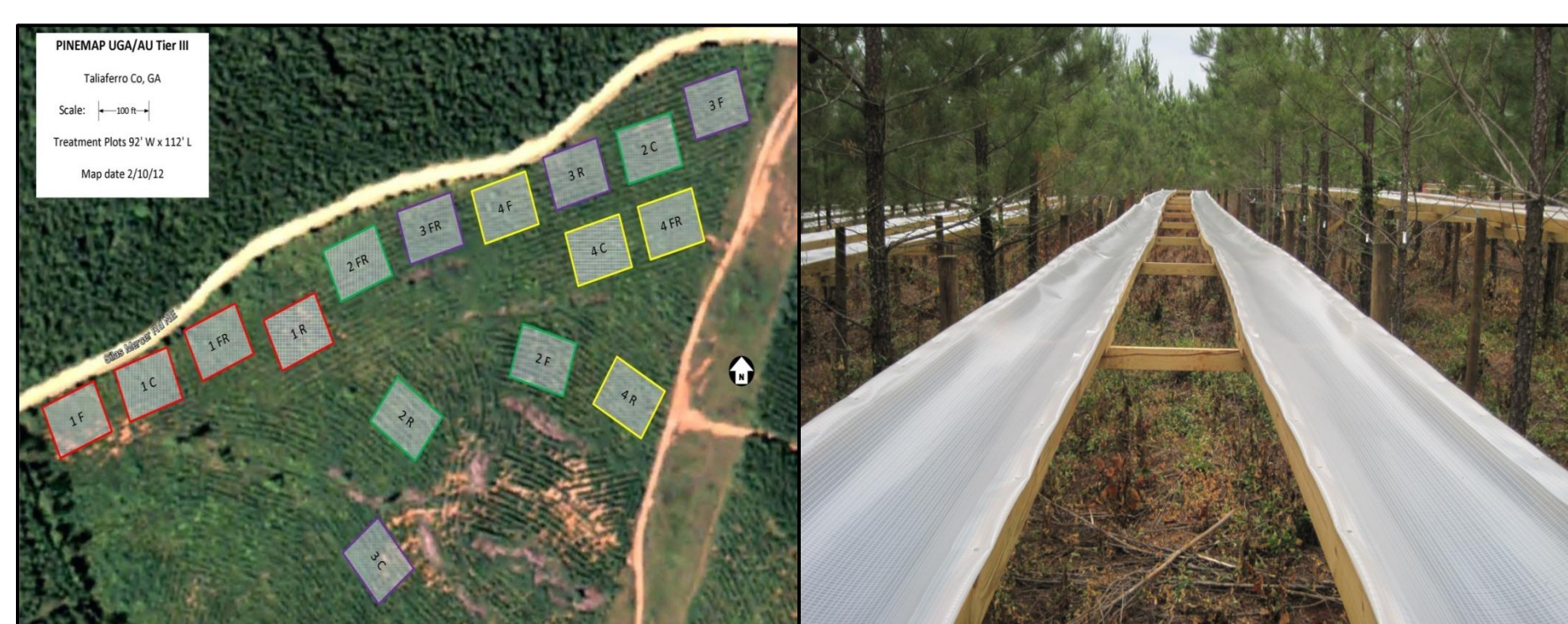
Fig. 1 (above left) Experimental treatments and blocks for a throughfall exclusion study in 8-yr-old loblolly pine plantation in Taliaferro County, GA. Note blocks (indicated by different colors) were established by tree height and basal area; (above right) Throughfall exclusion structure.
