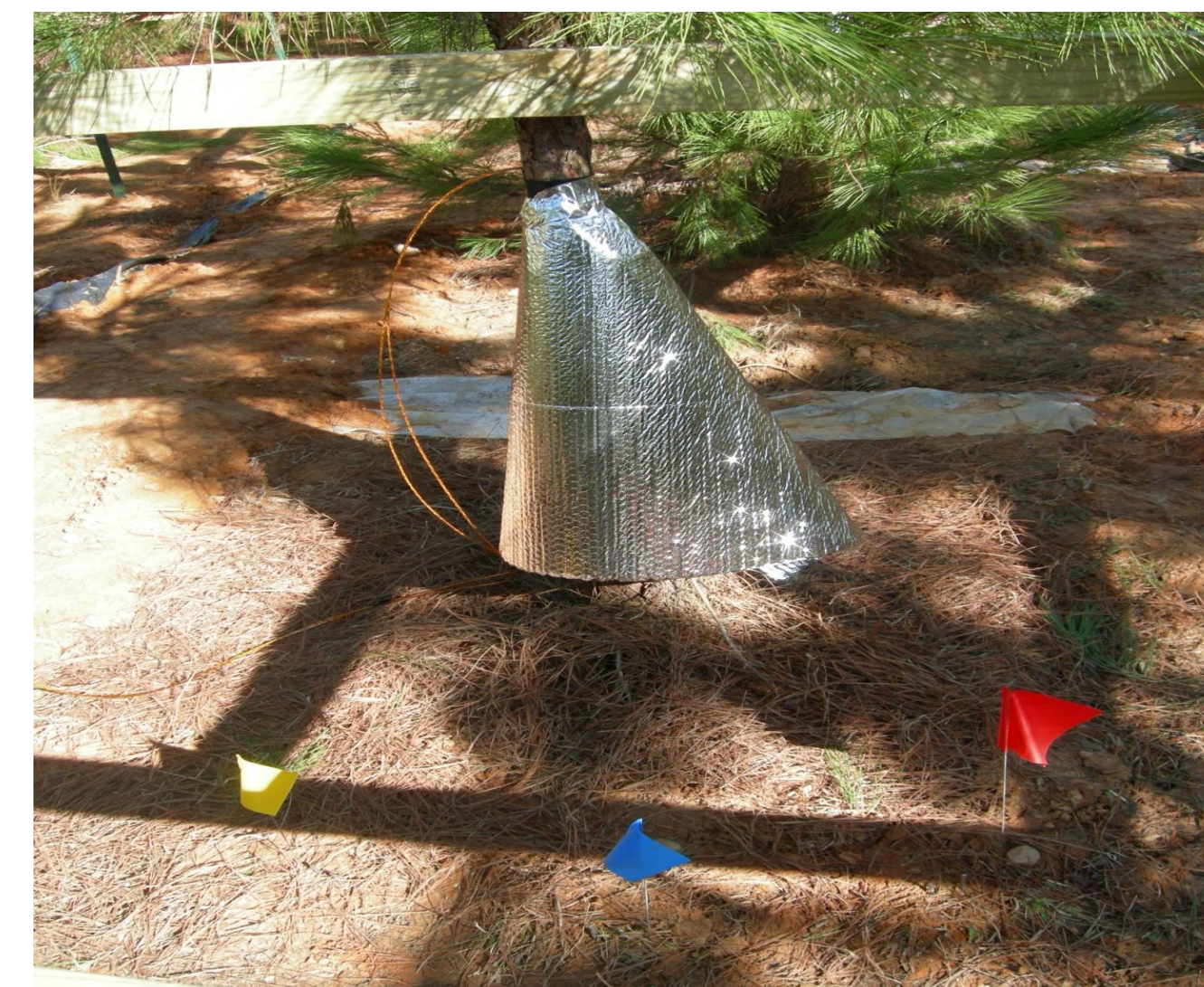
Figure 3. Thermal dissipation probes inserted and wrapped in a measurement tree, along with TDR rods at different depths in the soil.
