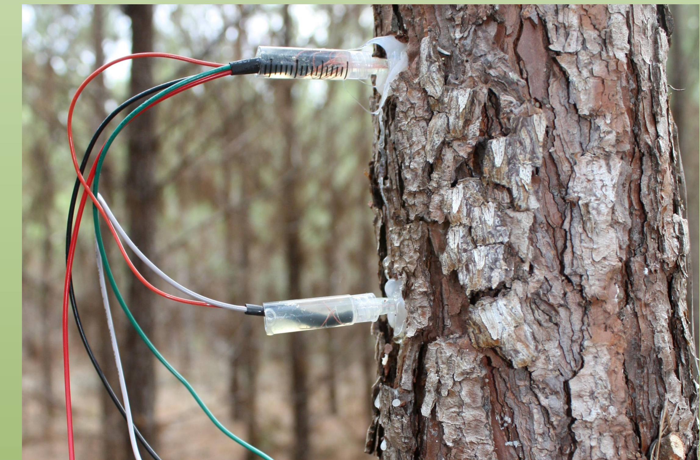
Figure 5. Sap flow probe in loblolly pine stem
