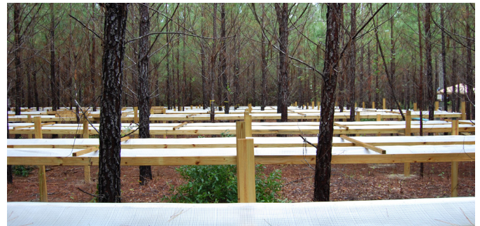
Figure 4. Throughfall exclusion structures at Tier III site in Taylor County, Florida. Photo by Geoffrey Lokuta.
