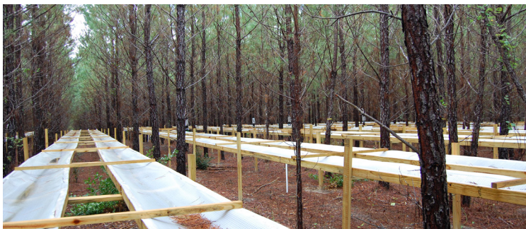
Throughfall exclusion structures at the PINEMAP “Throughfall Exclusion x Fertilization” site in Taylor County, Florida.
