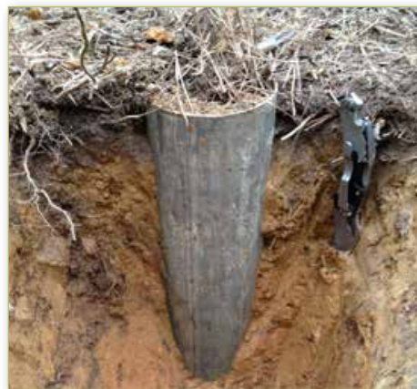
Figure 8.1. Right: Root-severing core installed at the Virginia Tier III site. Left: Root-severing core being excavated. Photos by Brett Heim.
