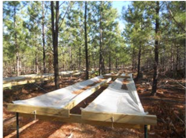
Figure 1c. Completed prototype of rain throughfall exclusion structure at Tier III site in Buckingham County, Virginia. Photo courtesy of Tom Fox.
