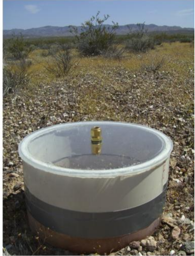
Figure 1 (Left). Schematic of a static chamber from Holland et al. (1999). Figure 2 (Right). A static chamber deployed in the field.
