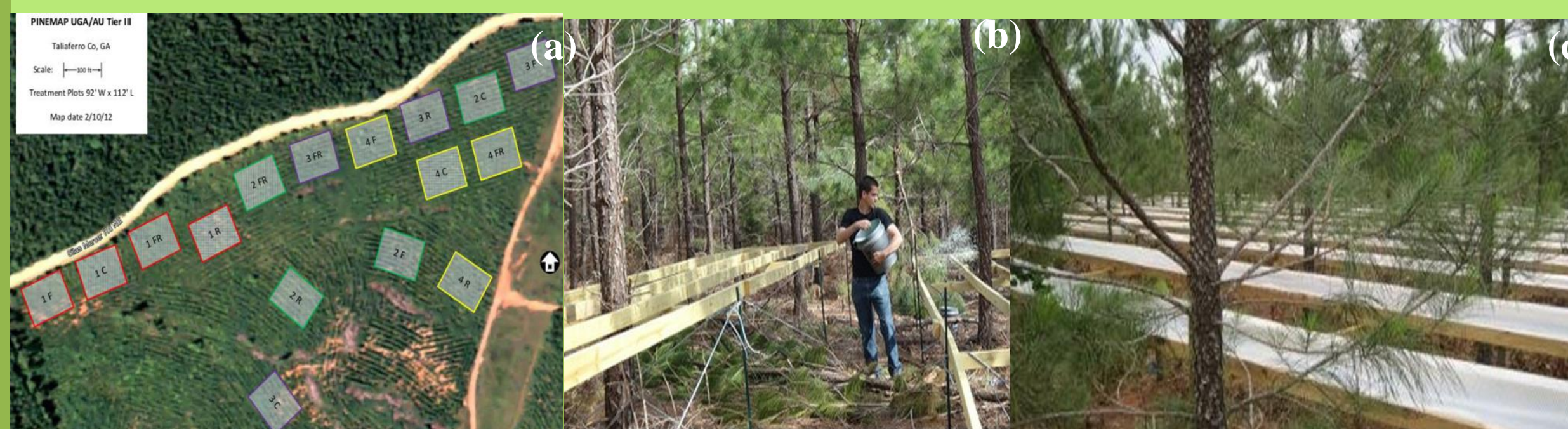
Fig 1. Map of Washington, GA Tier III site treatments (a). Different blocks are represented by differently colored borders around plots. Fertilization treatment (b) and throughfall reduction (c).
