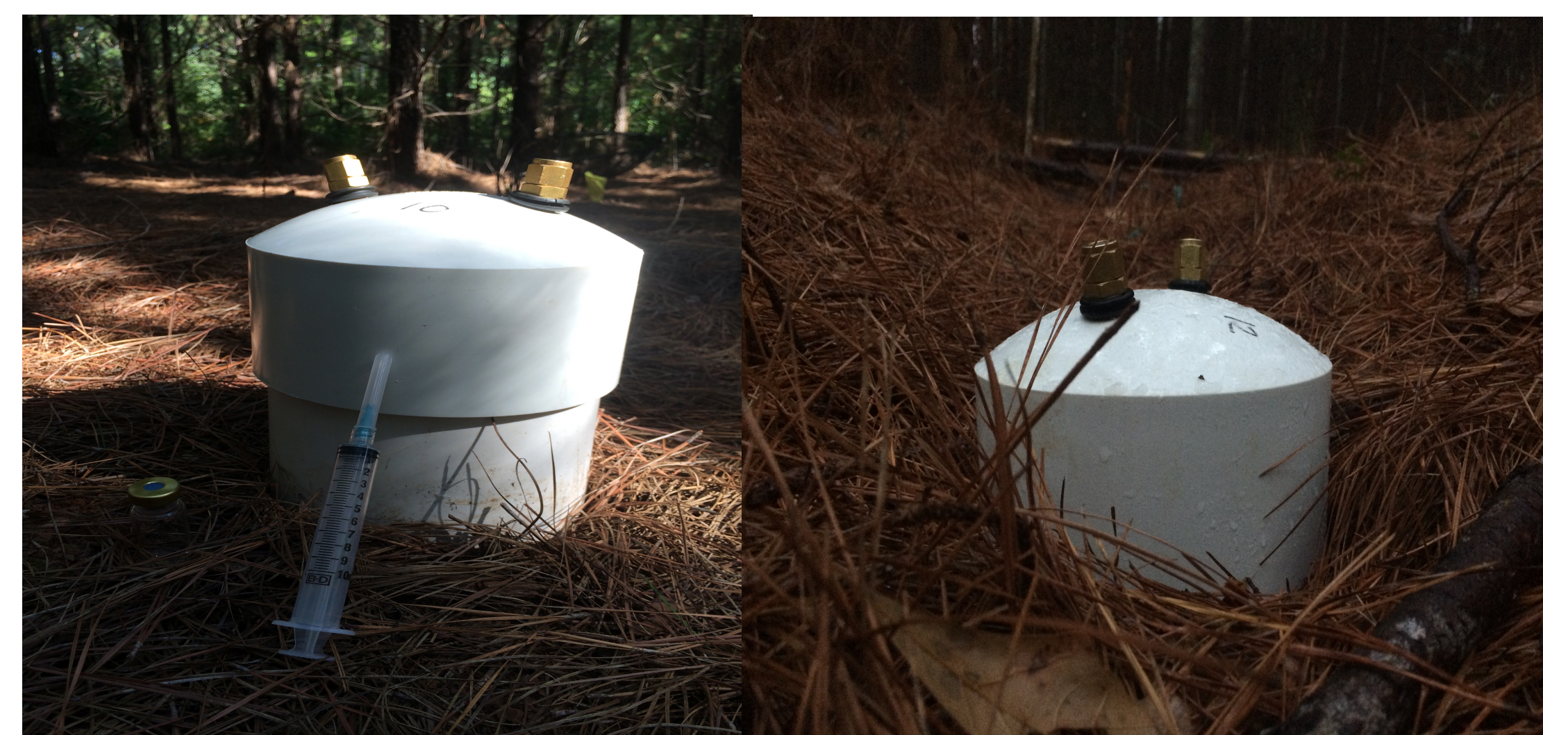
Figure 2. The static chamber approach was used to collect gas samples at 0, 10, 30, 50, and 70 minutes. Chambers are PCV pipe (6in X 5in) with a vented cap and septa for sampling with 10 mL syringe.
