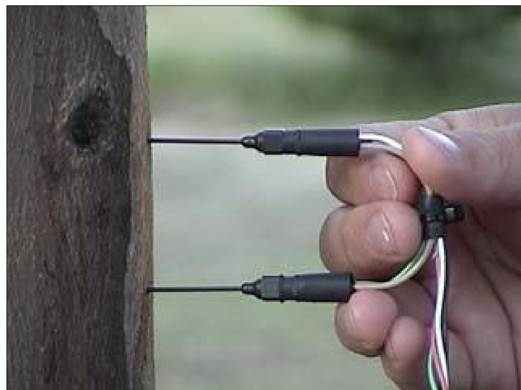
Figure 1. Schematic of Thermal Dissipation Probe sensor technology
