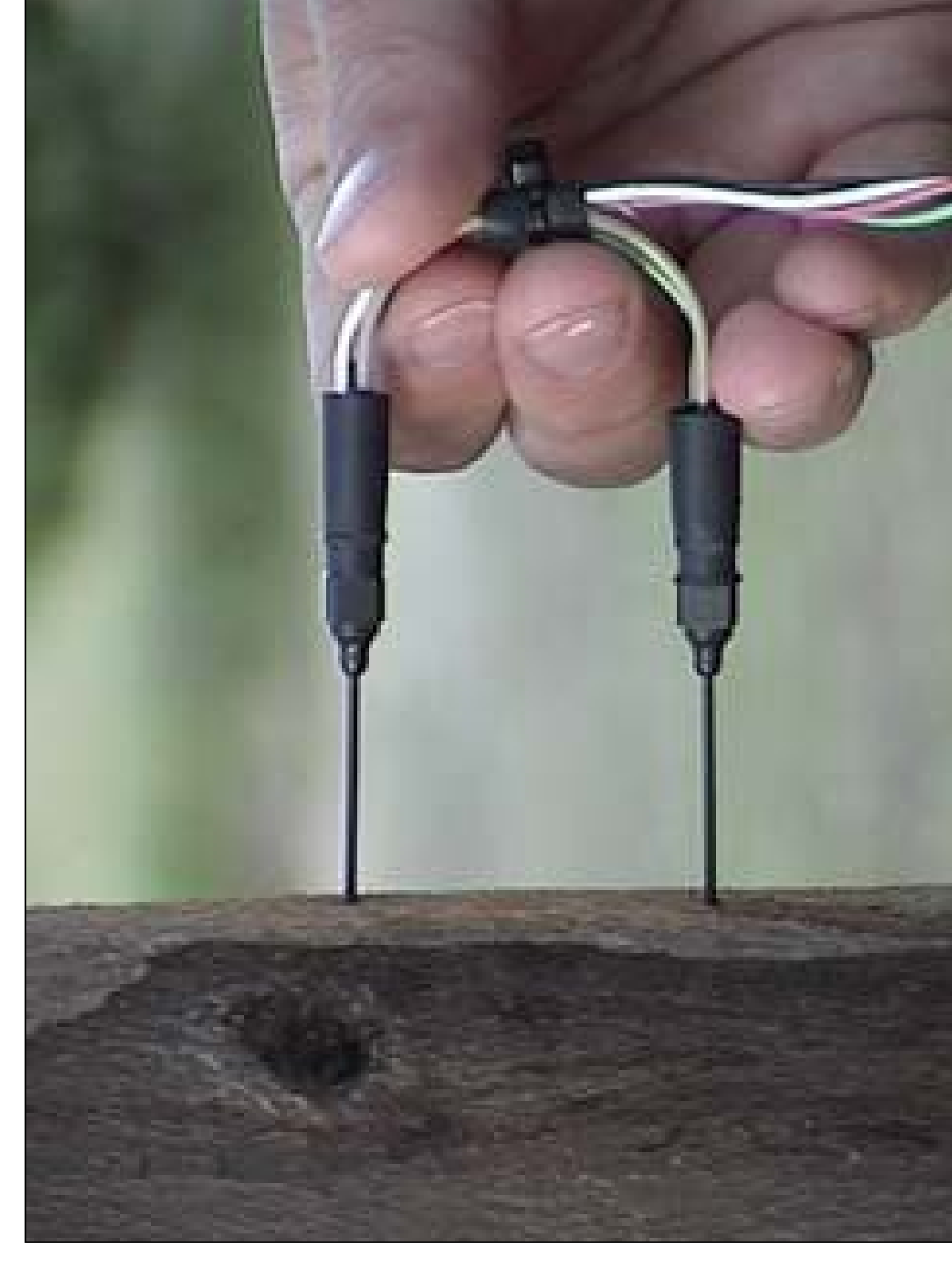
Figure 1. Schematic of Thermal Dissipation Probe sensor technology
