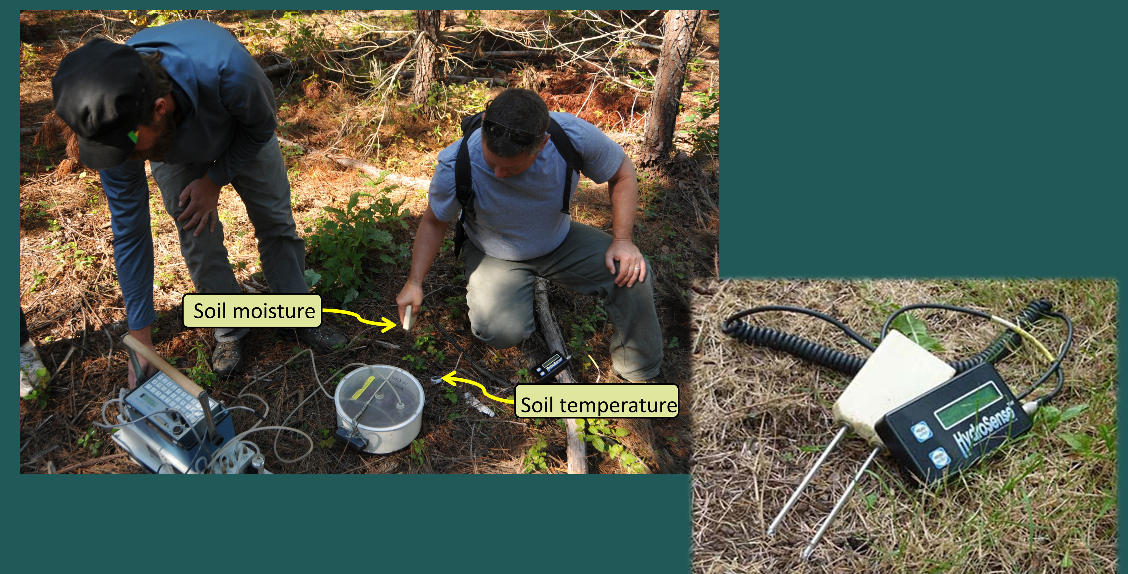
Figure 4. Soil moisture and temperature are measured at each sampling point. These measures are used to standardize soil CO 2 efflux rates.
