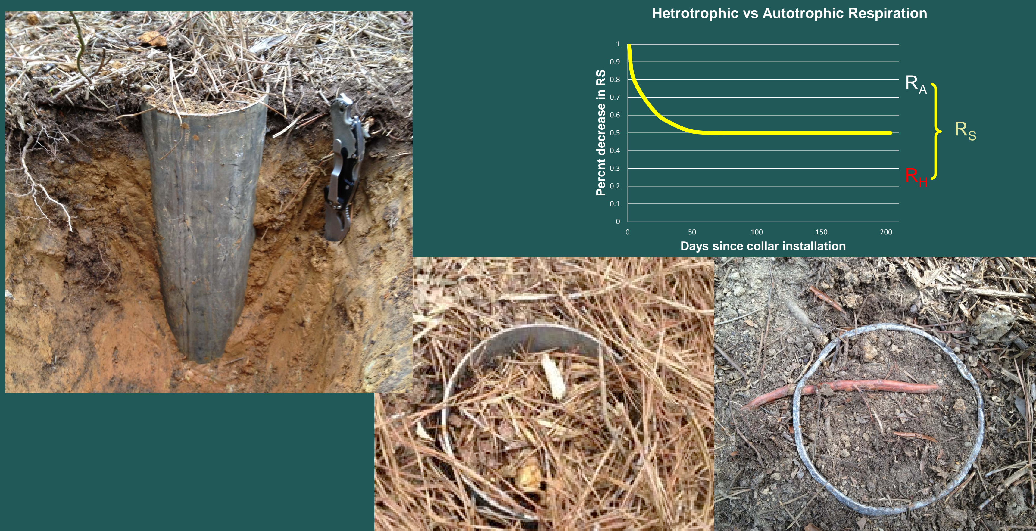
Figure 2. Installation of root isolation cores. Over time, respiration of roots in the chamber falls to zero and CO 2 emissions at this point are from soil heterotrophic organisms only (R H ).
