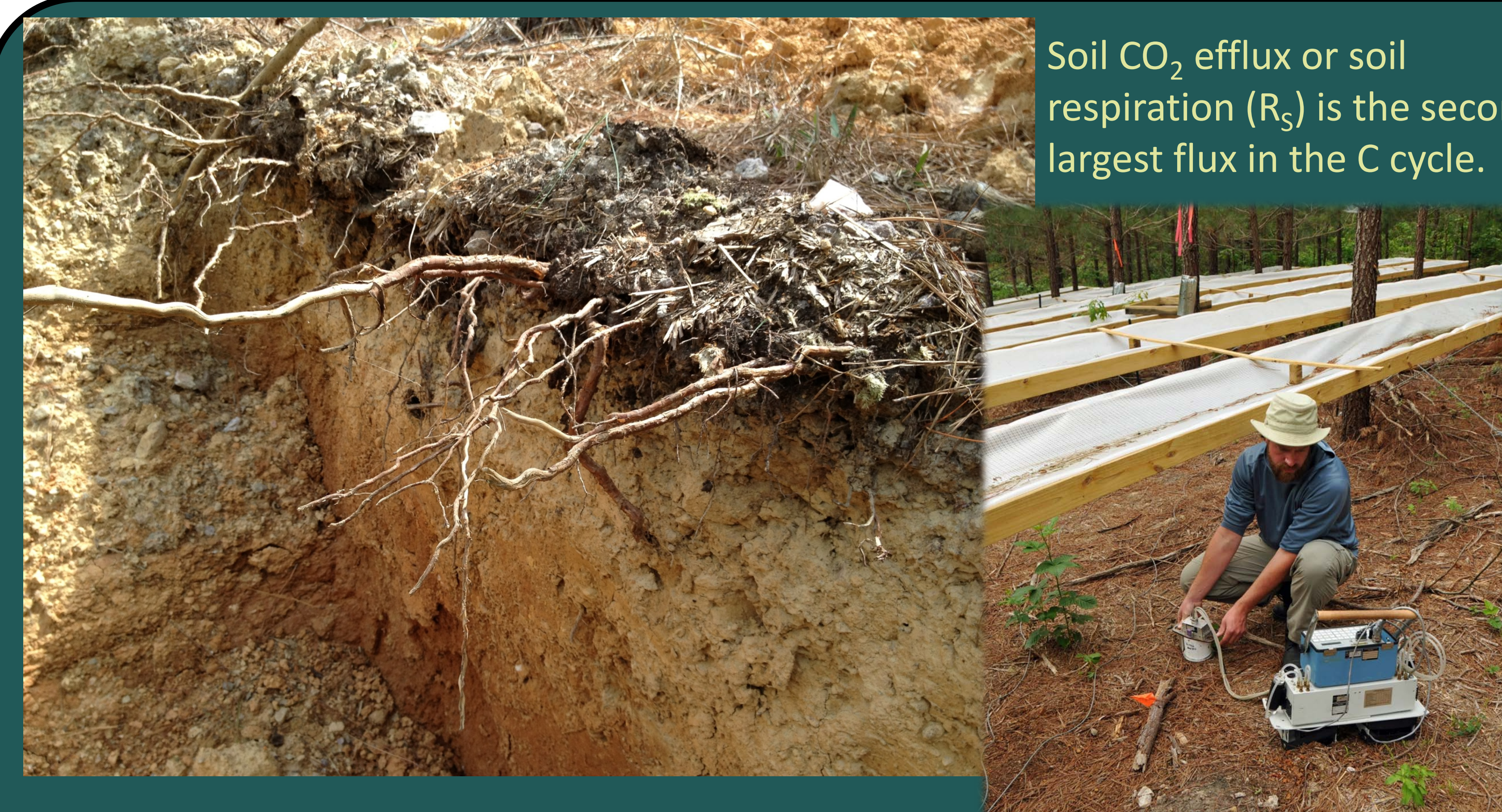
Figure 3. Soil CO 2 efflux is measured with a chamber sealed over the soil surface and an infrared gas analyzer. Measurements are taken over root isolation cores (R H estimate) and adjacent to cores (R H plus R A )
