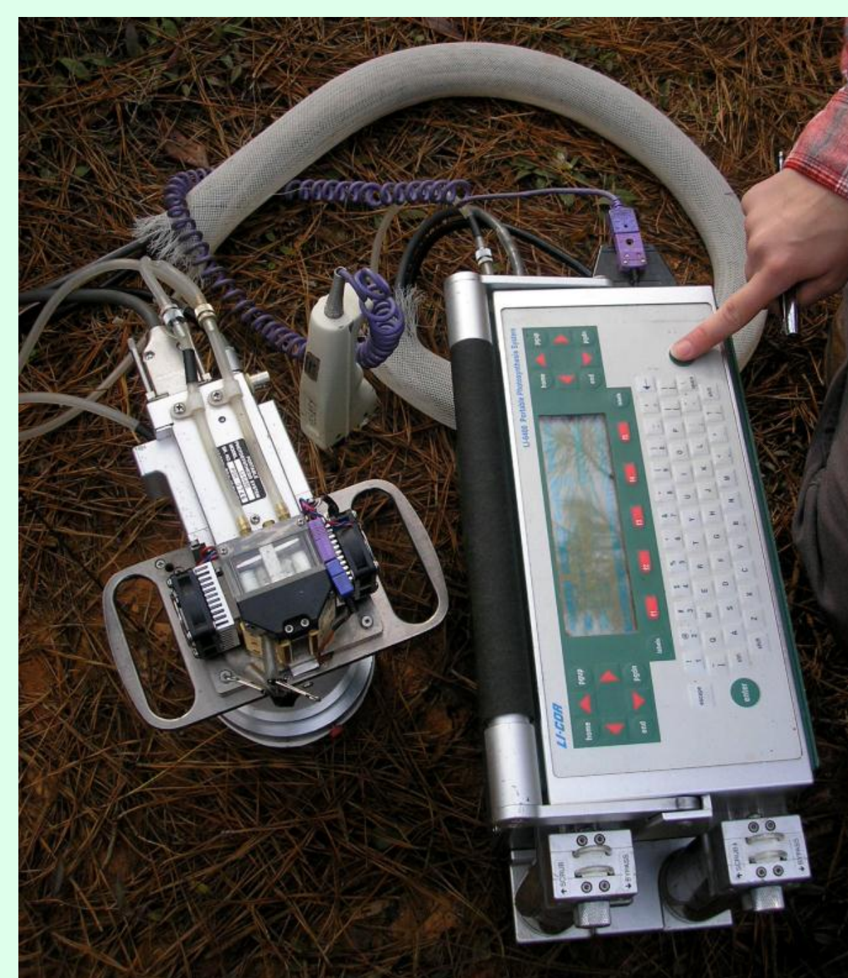
Figure 1: Li-6400 with soil chamber.
