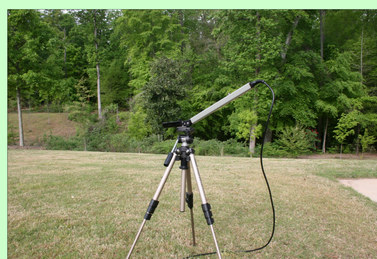
LAI 2000 in an open area taking automatic readings.
