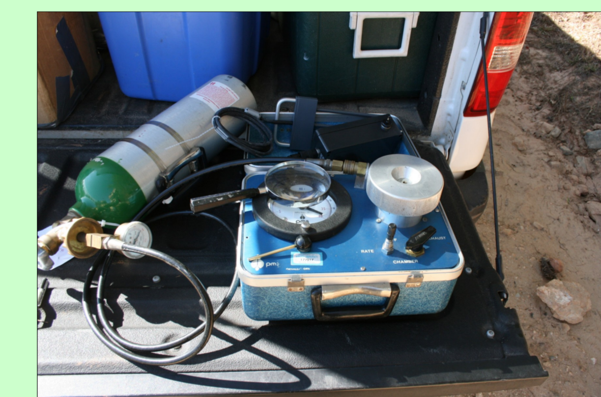
Pressure chamber used to measure water potential.
