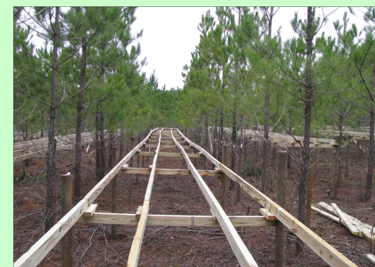
Rain exclusion trays that have been installed on the GA Tier III site.
