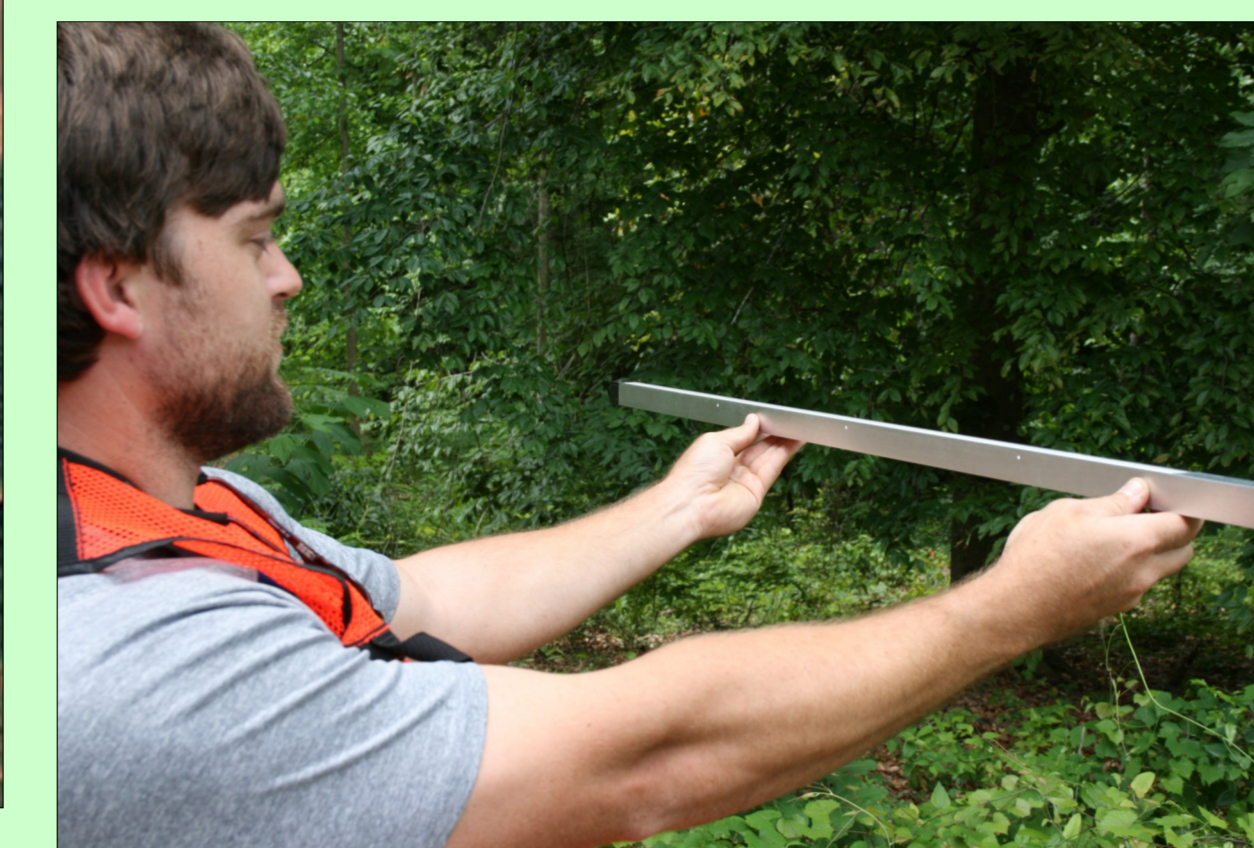
Measuring IPAR using ceptometer.
