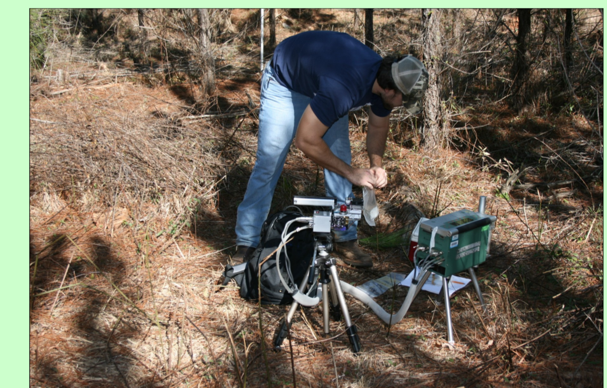
Measuring gas exchange with LICOR 6400.
