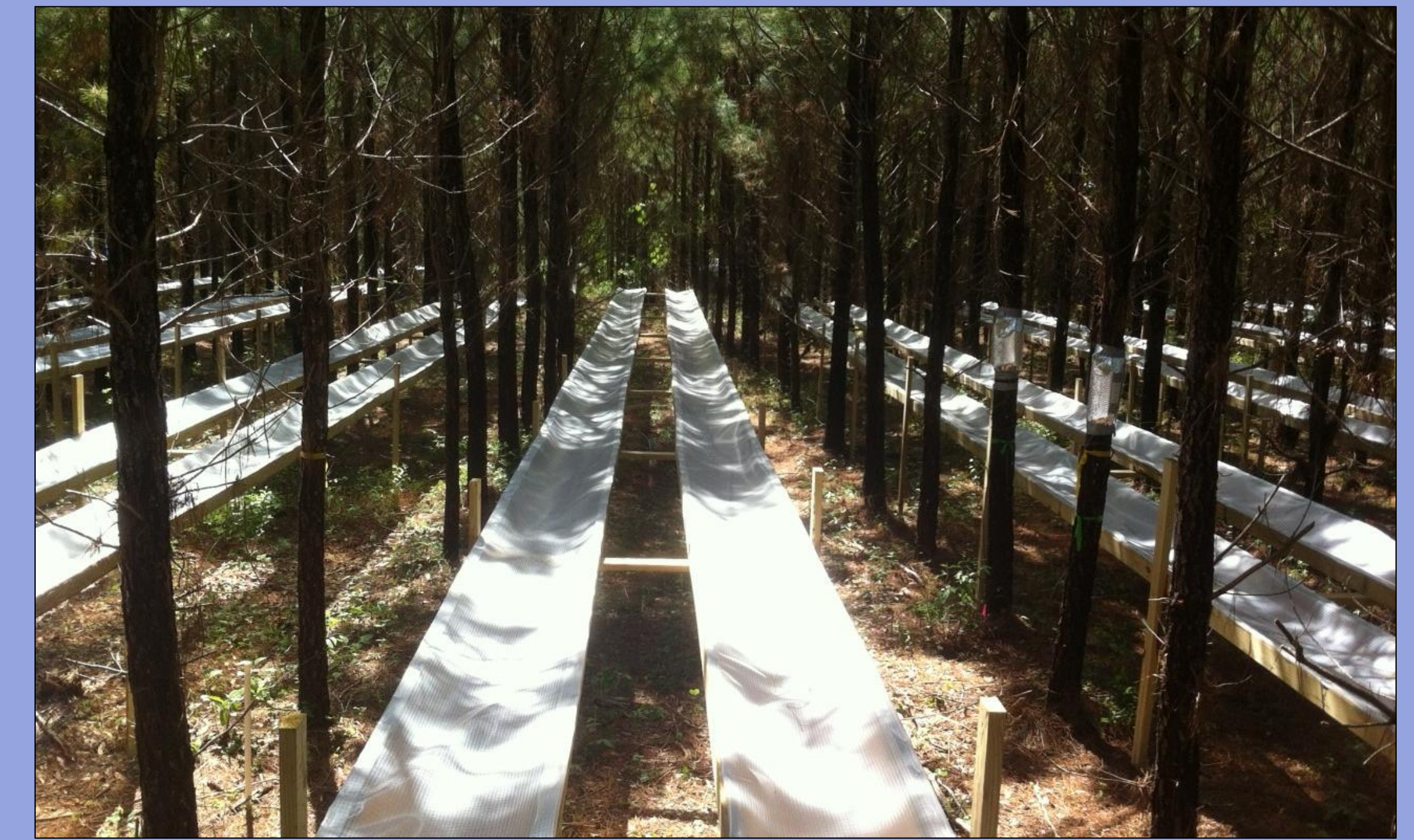
Rain throughfall exclusion structures erected below the canopy using pressure treated wood and clear extrusion laminated reinforced film.
