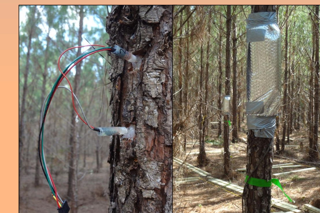
Sap flow sensors used to measure tree water use.
