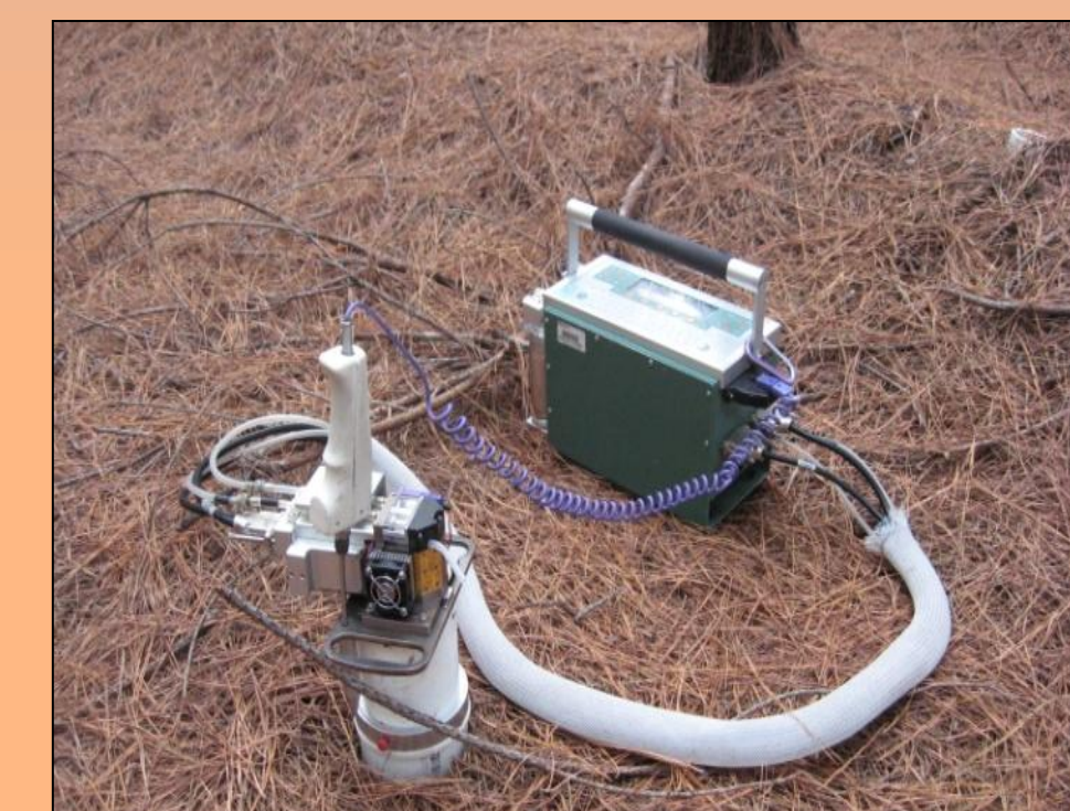
LI-COR 6400 infrared gas analyzer used to measure soil CO 2 efflux.
